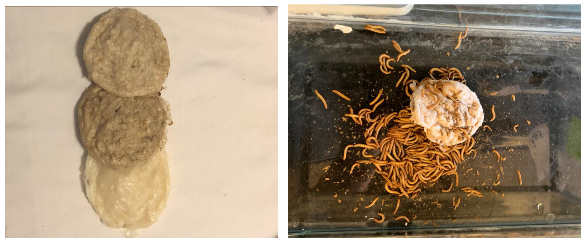
Figure 1- Pictured to the left are the results of the melting of the polyethylene. The top disk is oatmeal plastic, the middle disk is cornmeal plastic, and the final disk is plain plastic.
